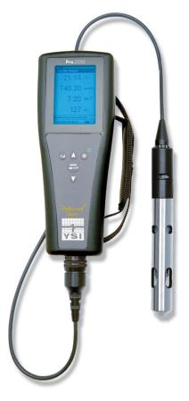
Parameters: Conductivity Specific Conductance Salinity Total Dissolved Solids (TDS) Dissolved Oxygen Temperature
